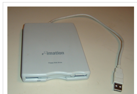
Imation USB Floppy Drive, model 01946. An external drive that accepts high-density disks.
