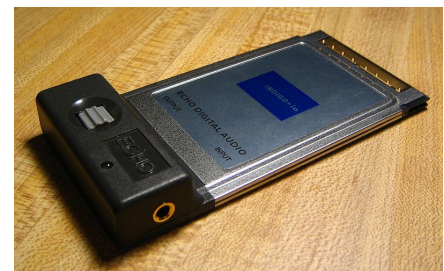
Echo Digital Audio Corporation's Indigo IO — PCMCIA card 24-bit 96 kHz stereo in/out sound card.
