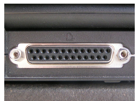
A DB-25 parallel printer port, as on IBM-PC style, and a few other types of computers.
