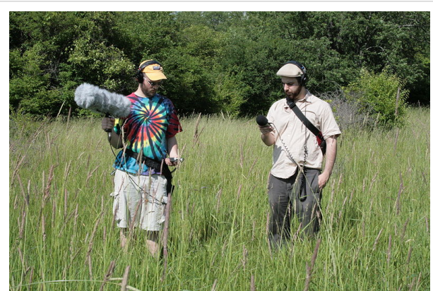
Two recordings being made—A blimp is being used on the left. An open-cell foam windscreen is being used on the right.
