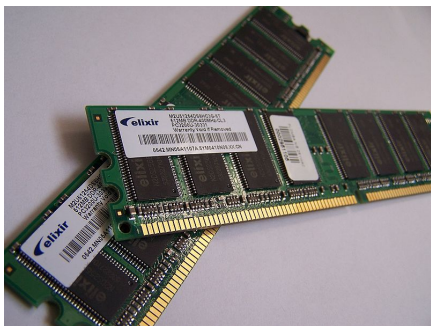
Example of writable volatile random-access memory: Synchronous Dynamic RAM modules, primarily used as main memory in personal computers, workstations, and servers.
