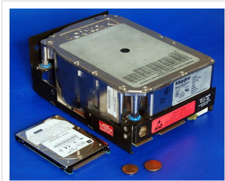
5¼" full height 110 MB HDD, 2½" (8.5 mm) 6495 MB HDD, US/UK pennies for comparison.
