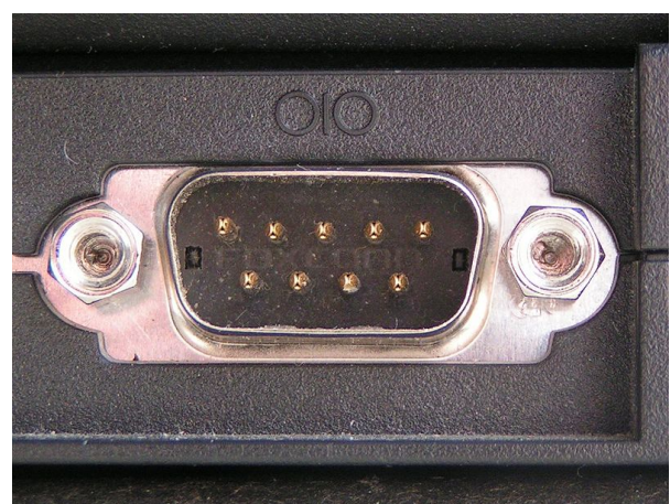
A male DE-9 connector used for a serial port on a IBM PC compatible computer. (Pinout)
