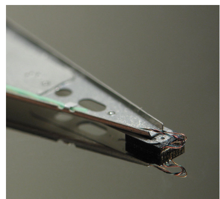
Close-up of a hard disk head resting on a disk platter. A reflection of the head and its suspension is visible on the mirror-like disk.
