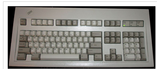
The PS/2's Model M keyboard from which modern PC keyboards are derived
