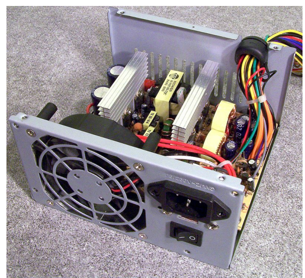
The top cover has been removed to show the internals of a computer Power supply unit.
