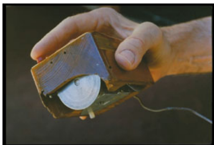
The first computer mouse, held by inventor Douglas Engelbart, showing the wheels that make contact with the working surface
