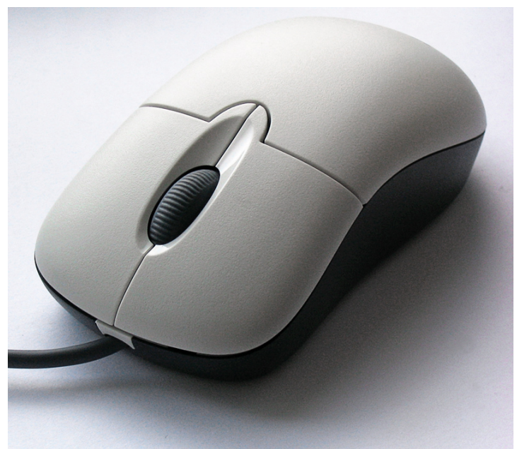
A computer mouse with the most common standard features: two buttons and a scroll wheel, which can also act as a third button
