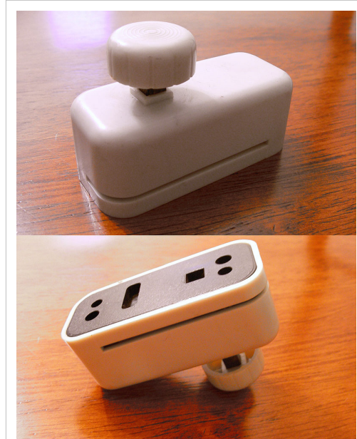
A disk notcher used to convert single-sided 5.25-inch diskettes to double-sided.
