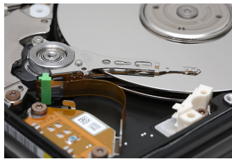
Interior of a hard disk drive
