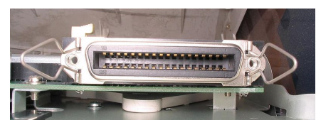
Micro ribbon 36 pin female, such as on printers and on some (particularly industrial and early- and pre-1980s personal) computers.
