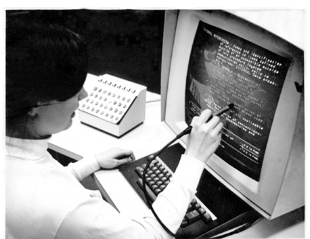
Photo of the Hypertext Editing System (HES) console in use at Brown University, circa October 1969. The photo shows HES on an IBM 2250 Mod 4 display station, including lightpen and programmed function keyboard, channel coupled to Brown's IBM 360 mainframe.
