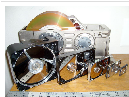
Six hard drives with 8", 5.25", 3.5", 2.5", 1.8", and 1" disks, partially disassembled to show platters and read-write heads, with a ruler showing inches.
